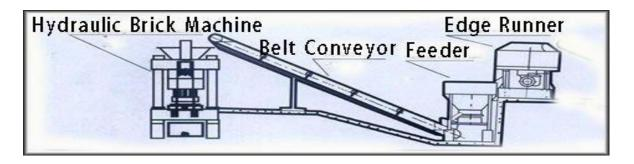
As you see in picture, edge runner, feeder, belt conveyor, brick machine consist of a simple production line.
